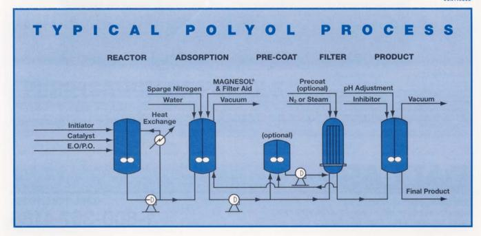
Following stripping, add the proper amount of water to the treatment reactor prior to increasing the temperature. The WET Method (Water Enhanced Treatment) is effective for optimizing the use of MAGNESOL® in some polyols.
